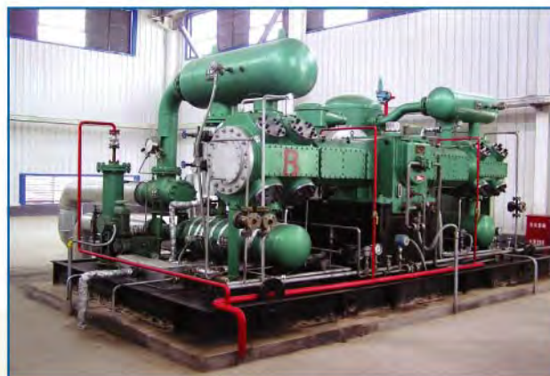
compressor with common skid
