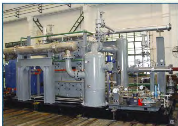
first set of 3-throws labyrinth piston compressor for 20 t/year polypropylene
