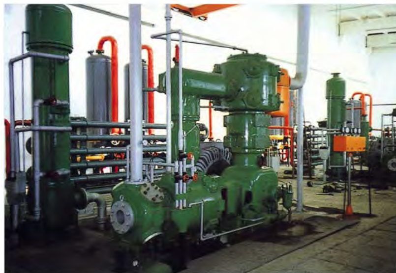
LW-4/8-X oil free piston air compressor unit (steel mill)
